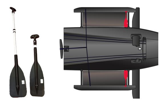
WARNING: It is generally strongly suggested to drop down both foils when hoisting and dropping the mainsail in order to avoid damaging it with the foils trailing edges that are pretty sharp!
