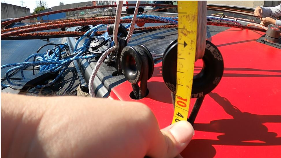
3. Once ensured that the mast is symmetrical, check the tension reading on the V1 shrouds is between the values listed in the table below for step 1. As a general guideline, the
