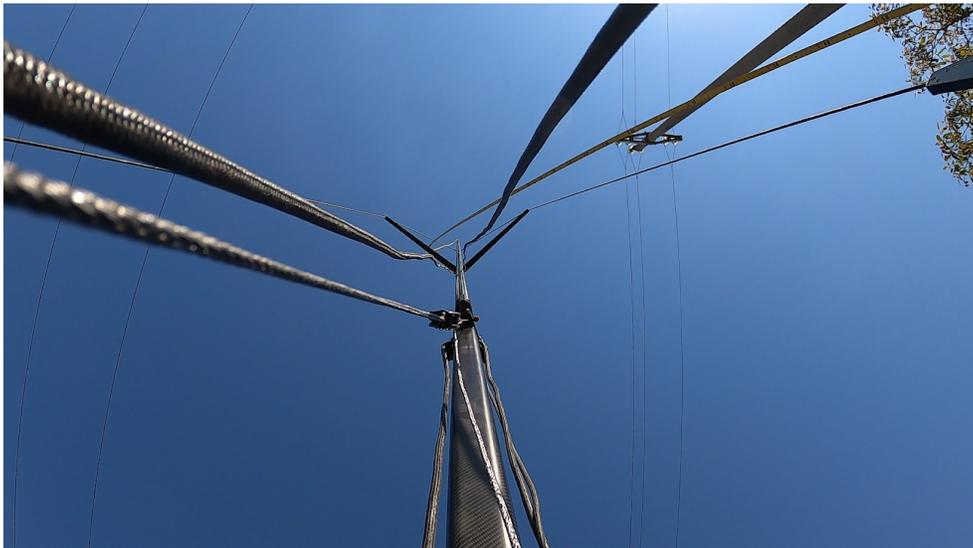
6. Once ensured that the mast is symmetrical, check the tension readings on the V1 and D2 shrouds are between the values listed in the table below for step 2.
