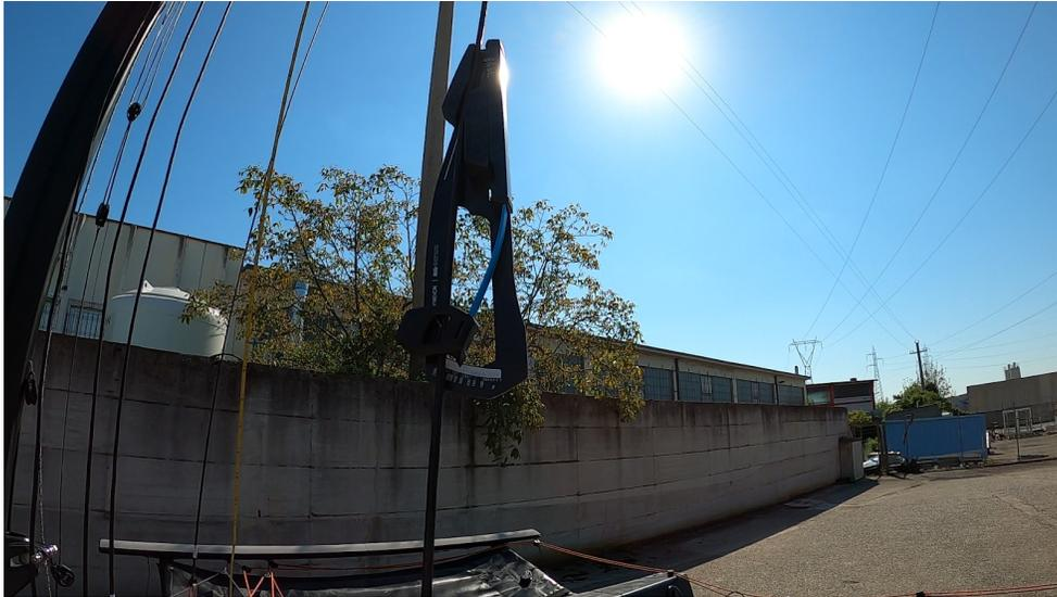
4. Release the tension on the forestay tensioner until it is possible to make three loops with the D2 Anacondas around the aftmost Ropeye.
