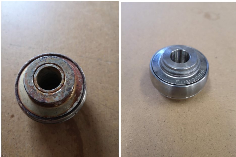
Bottom bearing before (left) and after (right) derusting.
