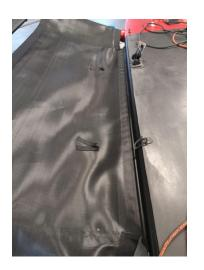
Pass the gennaker sheet block's soft shackle through the cut in the net.
