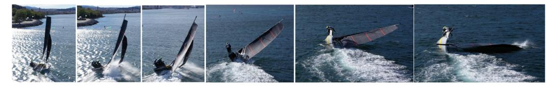
The racks are also slowing down the capsizing therefore usually the crew has some time to move up to the boat's side without going into the water.
