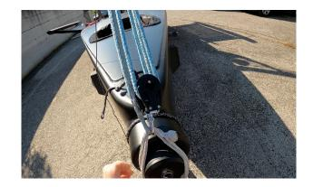
Pass the tensioner's soft loop around the bowsprit and pull the bowsprit out for safety. Make sure the purchase is completely eased off before doing so.
