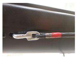
Before attaching the forestay, cow-hitch the spliced end of the jib halyard to the forestay top fitting. The jib halyard running outside of the mast is 2:1.
