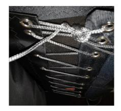
The rack seat cover is to be used during transport and storage as well as at the dock as a fender. The cover should be used at all times while at dock to avoid the rack seat and antiskid to be damaged in case of contact with other boats or with the dock itself.
